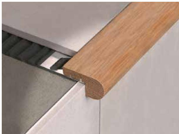
STAIRTEC FW is a stair nosing profile with a solid oak tread nosing inserted into a perforated aluminum base designed to be adhered into the bonding mortar. Its simple, traditional wood stair design can be used in both modern and traditional settings. Particularly ideal for residential applications, STAIRTEC FW can even be used for edging tiled kitchen countertops.
